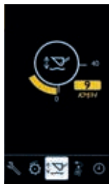
Adjustable SRS engagement speed.
